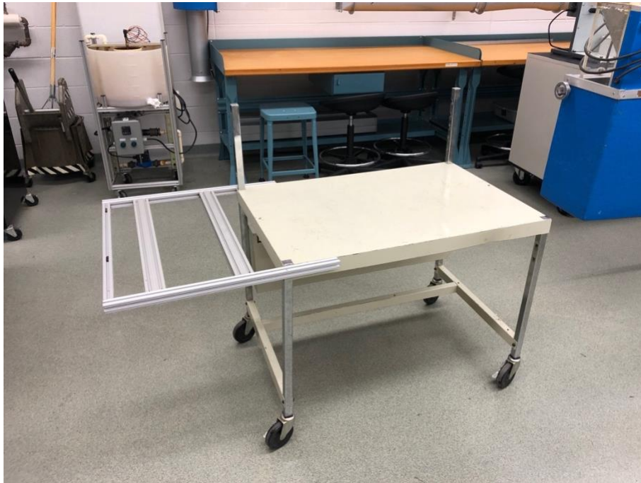
Figure 1: Cart After the 80/20 Extension was Added
