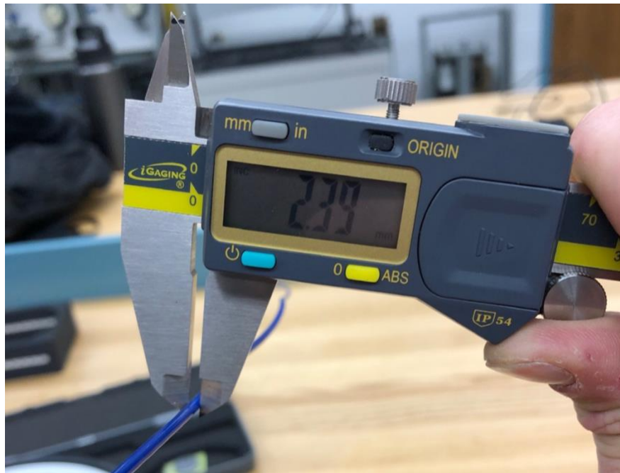
Figure 50: Extruded Filament above Target Diameter
