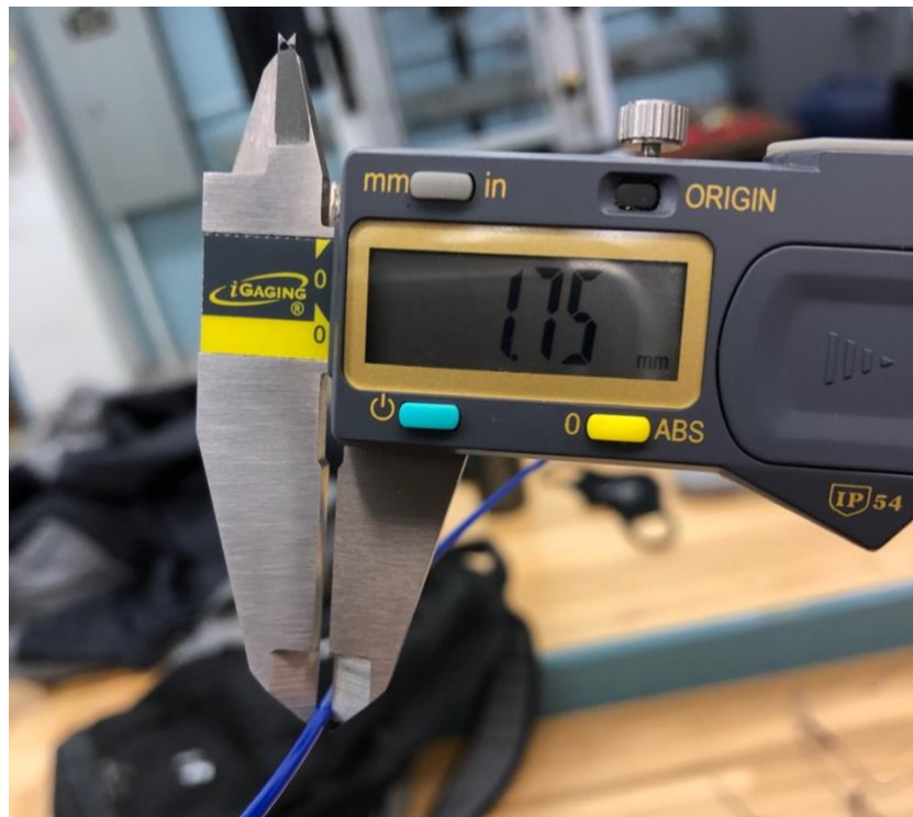
Figure 49: Extruded Filament at Target Diameter
