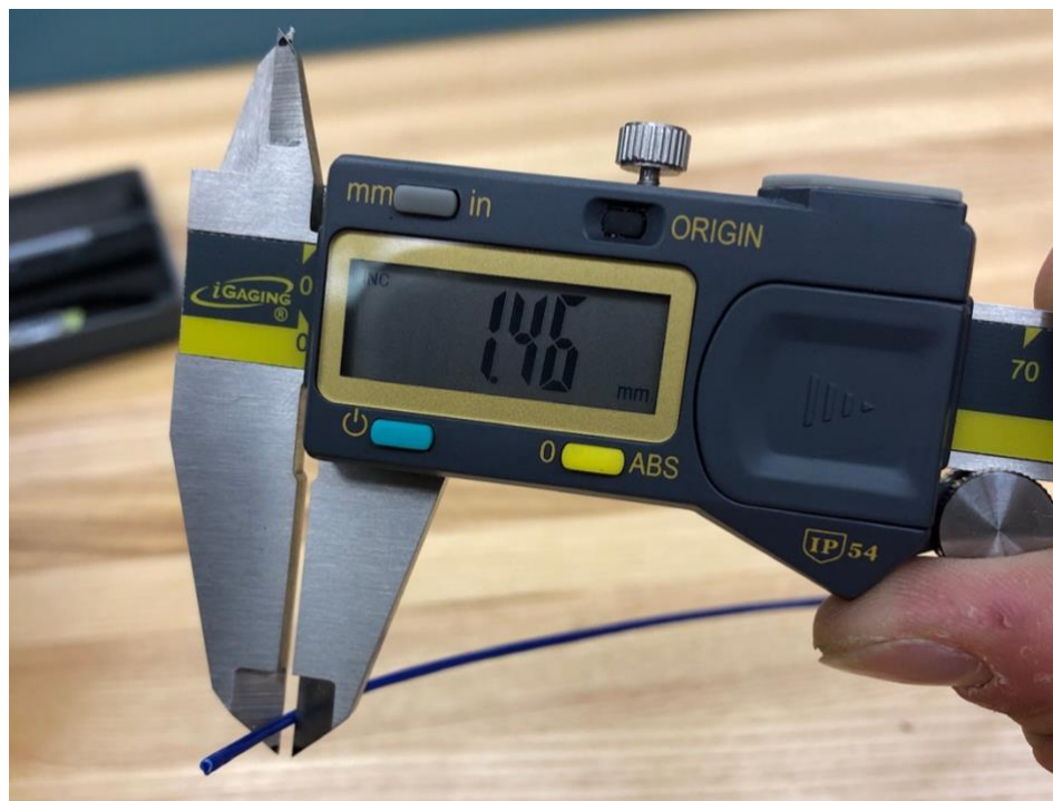
Figure 51: Extruded Filament below Target Diameter
