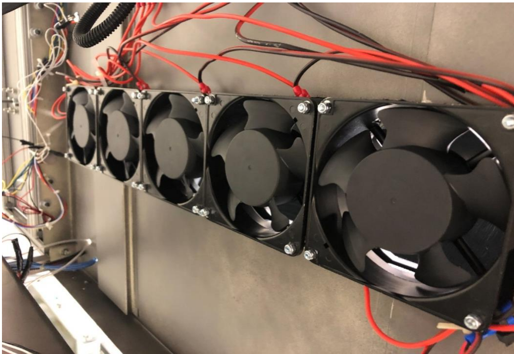
Figure 19: Bottom View of Duct and Fans Inserted in the Cart
